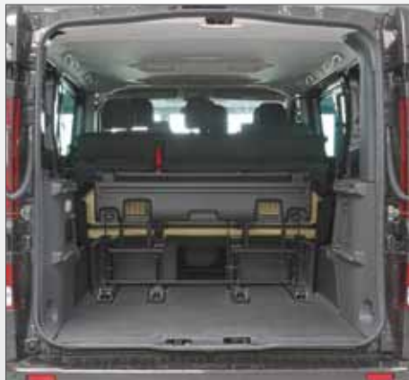
Third-row bench covers and wheel arch covers. The lower covers are designed to be tilted, easing the storage of long equipment.
